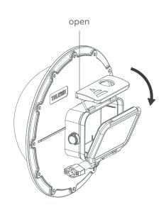
2. Put the camera and anti-fog insert in. Close the back door and lock it.
